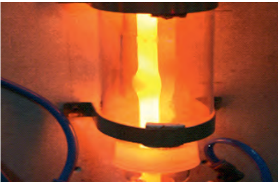
Fig. 17: Clad High Temperature Burst and Thermal Shock Shattering Tests. These tests are required to arrive at fuel failure criteria following design basis and postulated severe accidents in nuclear reactors. The above tests are for clad of Indian PHWRs. High temperature tests (up to 1200°C) are for simulating power rise following Loss of Coolant Accidents (LOCA) and shattering tests are to assess clad structural integrity under thermal shock following cold injection of water from Emergency Core Cooling System (ECCS). Till date more than 200 numbers of such tests have been performed. These studies formed basis of Indian clad specific failure data required for severe accident safety assessment
