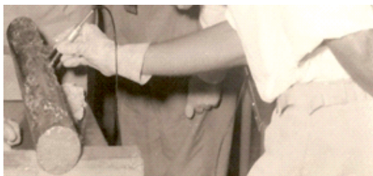
Fig. 7(b): Left Picture -Ultrasonic Testing (UT) of uranium billet for CIRUS Fuel. Right Picture-Eddy Current testing (ECT) of CIRUS rod. These techniques were developed at a time when there was no know how of this subject, in Indian industry. Later experts from BARC took active initiative in disseminating knowledge gained in this field, to specialists of other industries.
