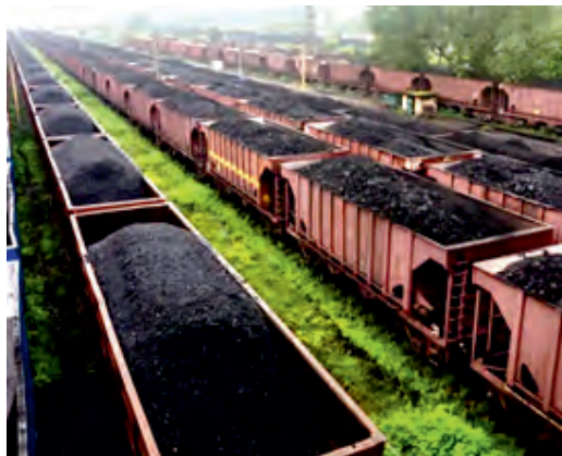
Fig. 2(b): Transportation of coal from mines to power station site is expensive and puts heavy demand on transportation infrastructure. A typical 500 MWe unit demands two 50 wagons goods train carrying 5000 tonnes of coal daily from mines to power station site. In the year 2021 about 700 million tonnes of coal was transported for different utility and captive power stations in India
