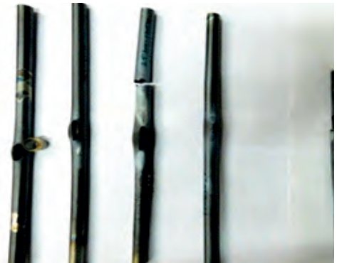
Fig. 17: Clad High Temperature Burst and Thermal Shock Shattering Tests. These tests are required to arrive at fuel failure criteria following design basis and postulated severe accidents in nuclear reactors. The above tests are for clad of Indian PHWRs. High temperature tests (up to 1200°C) are for simulating power rise following Loss of Coolant Accidents (LOCA) and shattering tests are to assess clad structural integrity under thermal shock following cold injection of water from Emergency Core Cooling System (ECCS). Till date more than 200 numbers of such tests have been performed. These studies formed basis of Indian clad specific failure data required for severe accident safety assessment
