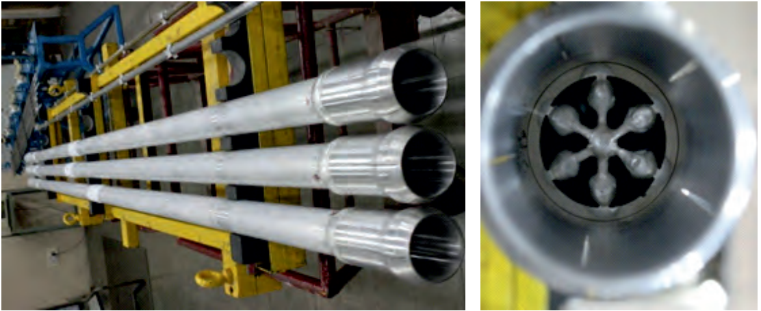
Fig. 10: Dhruva Reactor Fuel Clusters. Left figure shows the overall assembly (3 numbers of them are seen). Right figure shows end view of one of the assemblies. It is a cluster of 7 fuel pins. Dhruva fuel fabrication facilities are more or less identical to those of CIRUS fuel, shown in Fig.9
