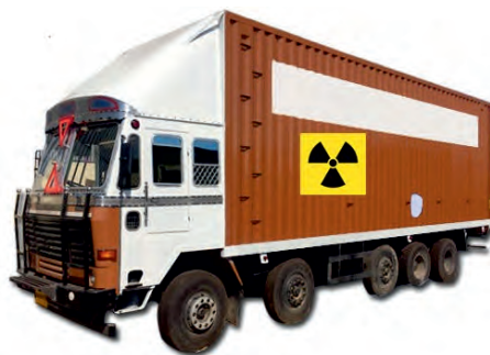
Fig. 3(b): Nuclear fuel is transported in trucks. 4 to 5 truck trips meet the annual nuclear fuel requirements of a typical 540 MWe Unit
