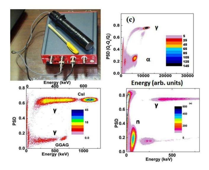
This invention describes a novel and the most versatile phoswich radiation detector consisting of two single crystals scintillators. It can detect and discriminate various types of radiations like alpha, neutrons, gamma simultaneously having versatile applications in academic, nuclear, security and medical fields. The detector has the highest figure of merit of discriminitation ability that is improved more than 100% when these single crystal scintillators are used separately
