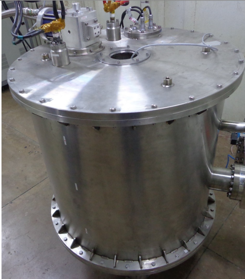
130mm diameter warm bore cryogen free magnet
