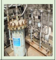
Pilot scale ion exchange system
