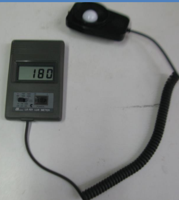
Lux meter, used for measuring light intensity (Illuminance measurement)
