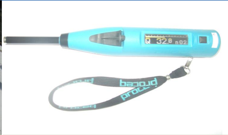
Rebound Hammer Tester for surface hardness checking of RCC structures
