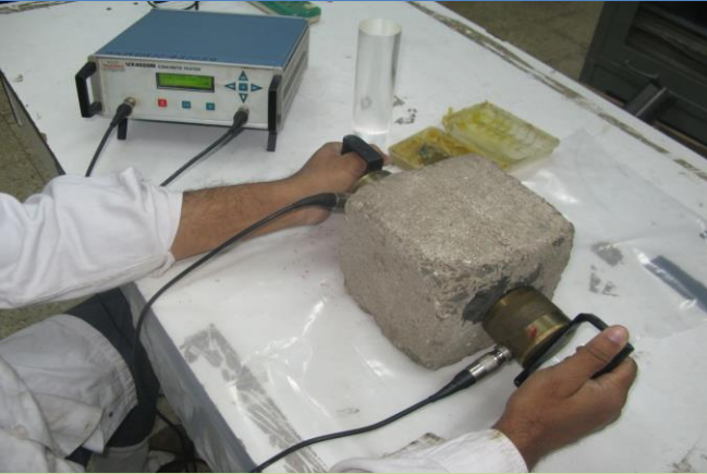
Ultrasonic Pulse Velocity (USPV) Testing Instrument for quality checking of an RCC structure
