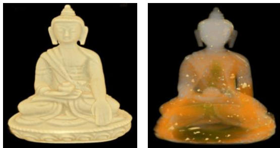
Neutron tomography of Buddha statue - (R) Wax remnants on surface due to bronze casting process detected
