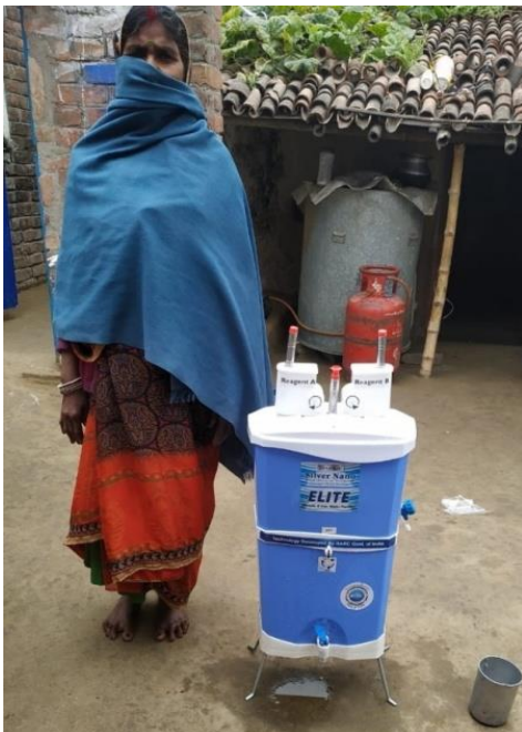
Point-of-Use arsenic removal device (24 LPD) installed at a household of Harail village, Bihar.
