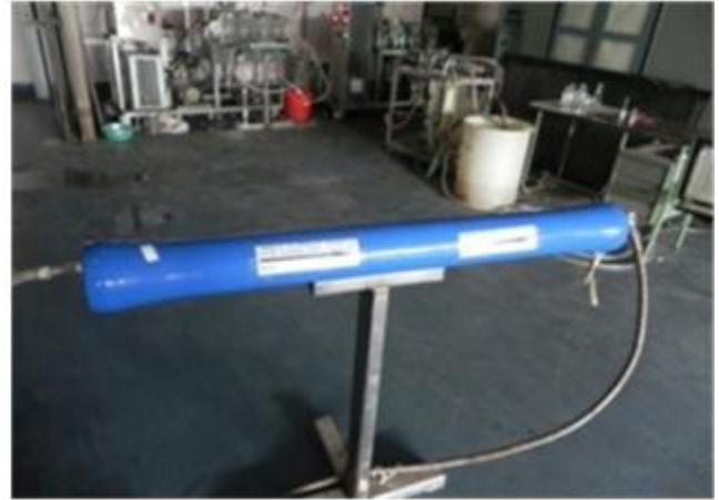
Spiral modules of charged nanofiltration membranes
