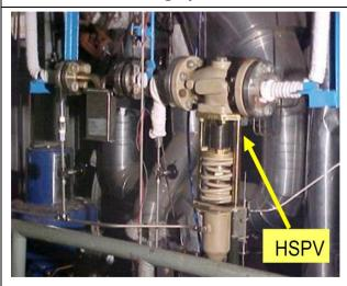
Testing of Hot Shut down Passive Valve
