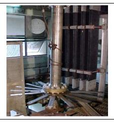
Electrically heated 54Fuel Rod Simulator used for Thermal Hydraulic Experiments
