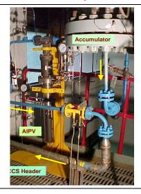
Testing of Passive Valve for injection of water from Emergency Core Cooling system
