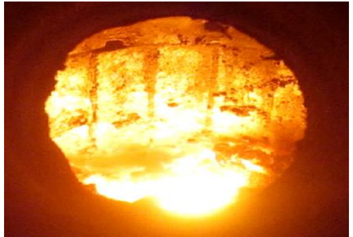
The extremely hot coke bed with bed temperature >1500°C
