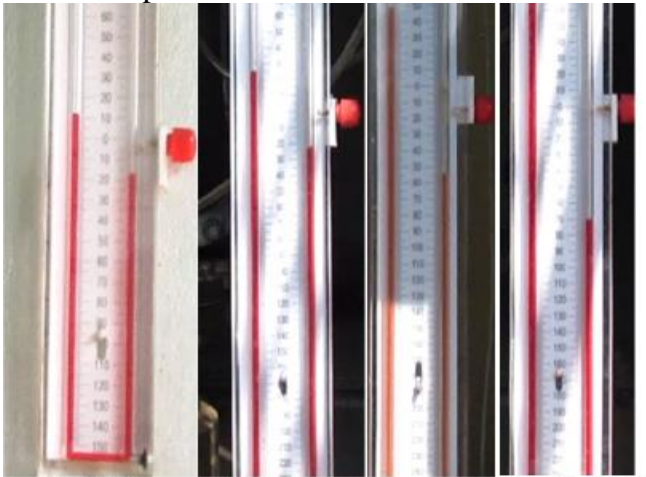
PRIMARY SECONDARY VENTURI PACKED BED Negative pressure maintained at different units
