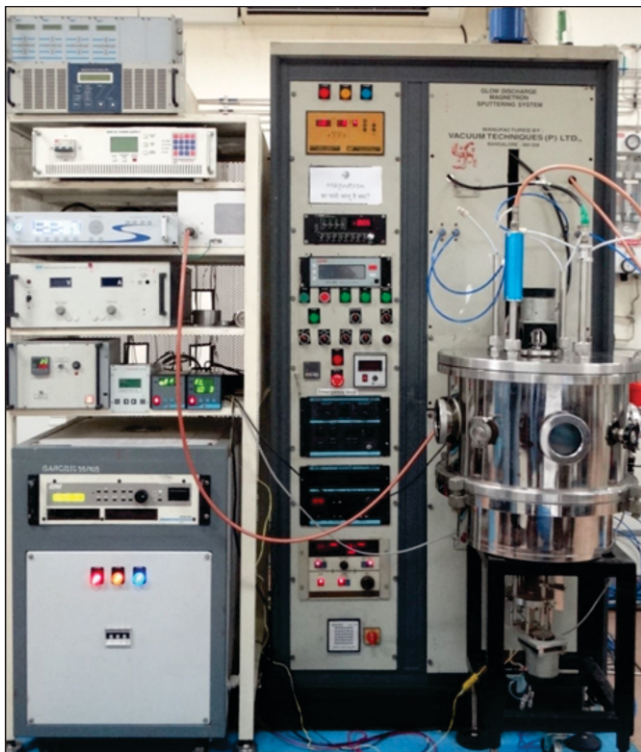
Fig.3: Unbalance DC/RF magnetron sputtering system used for Cr coating.
