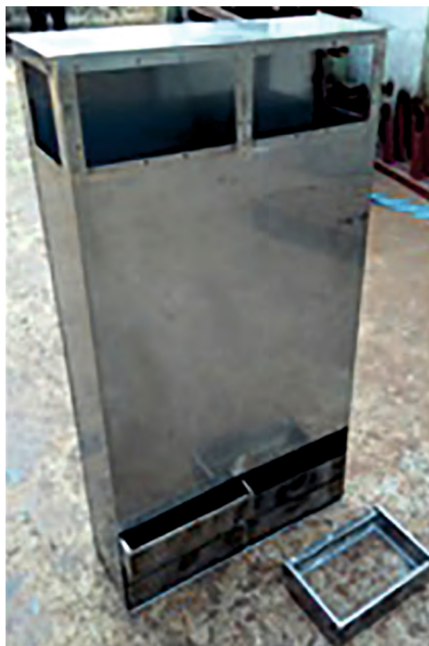
The Passive Catalytic Hydrogen Recombiner (PCHR) with Platinum and Palladium wire gauge catalyst bearing panels
