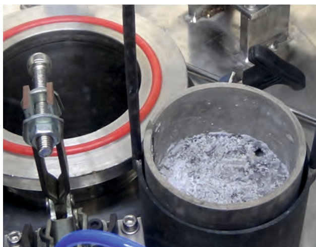
FLiNaK salt prepared inside molten salt corrosion test facility (MSCTF)
