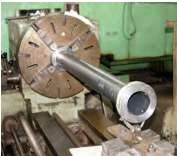
Facility for fatigue cycling test for 540 MWe Pressure Tube end fitting Rolled Joint
