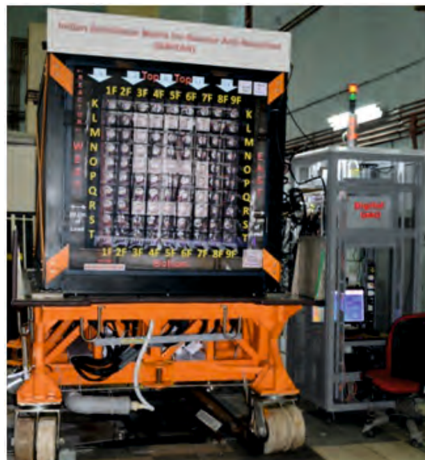
ISMARAN (Indian Scintillator Matrix for Reactor Anti-Neutrinos) detector setup at Dhruva Reactor
