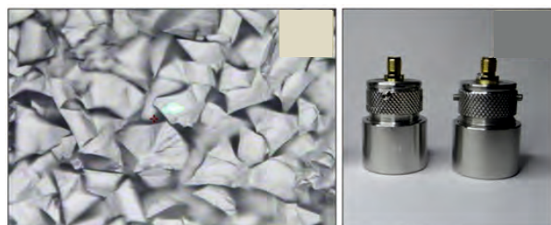
Large area CVD diamond films developed in BARC for optical and nuclear applications
