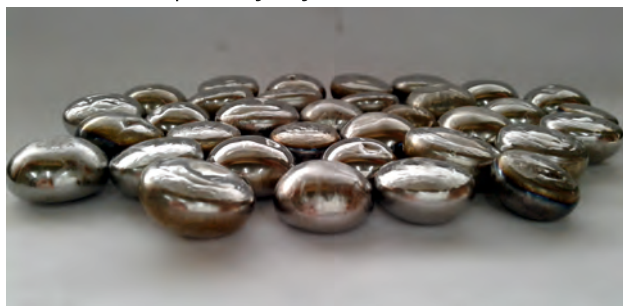
\text{Ti}_2\text{CrV} alloy samples synthesized for deployment in prototype hydrogen storage device
