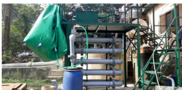
Compact helical shaped waste converter, Shesha, for biocomposting of waste
