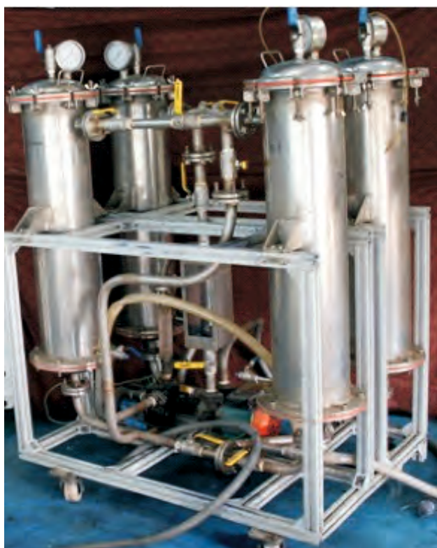
Community level purifier system for decontamination of Arsenic based impurities in water
