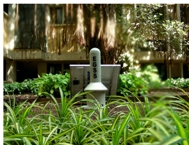
Environmental Gamma Spectrometry System (EGSS)
