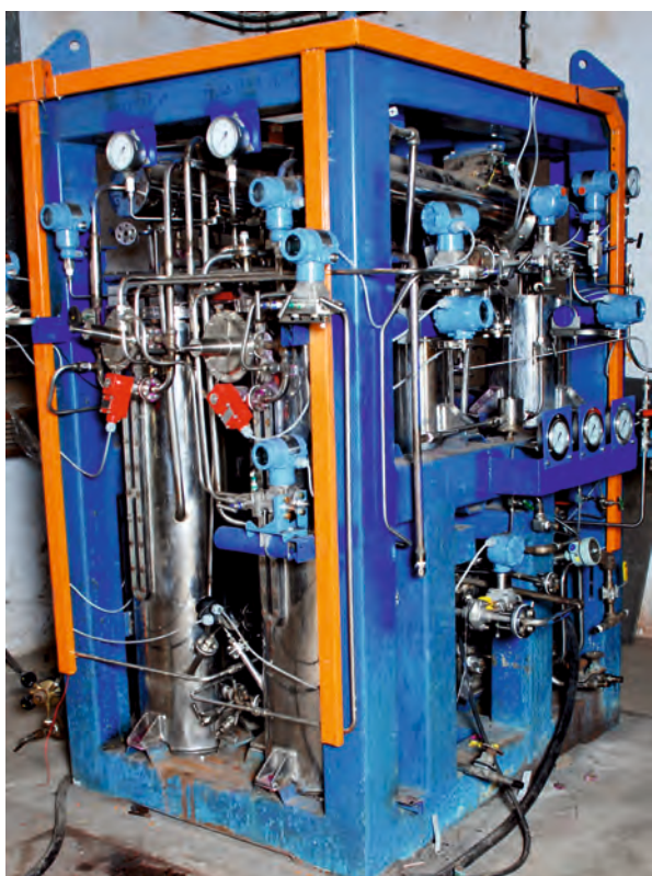
Alkaline Water Electrolysis Plant for production of Hydrogen and Oxygen
