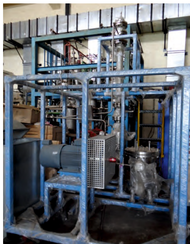
Pb-Li Extractor Loop showing high temperature electromagnetic pump
