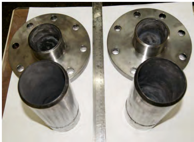
Aluminized (inner surfaces) SS 316 storage modules
