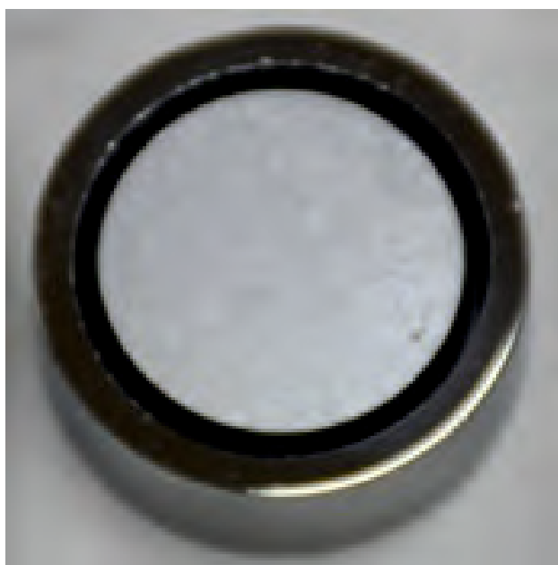
n-type HPGe detector fabricated in BARC
