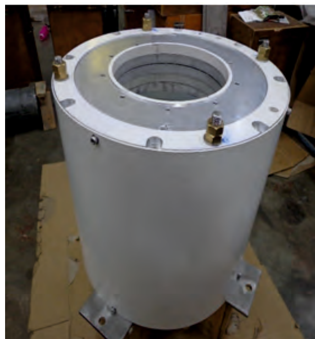
Halbach based permanent magnet dipole for imaging of specific body parts like head, wrist and ankle as part of primary diagnosis
