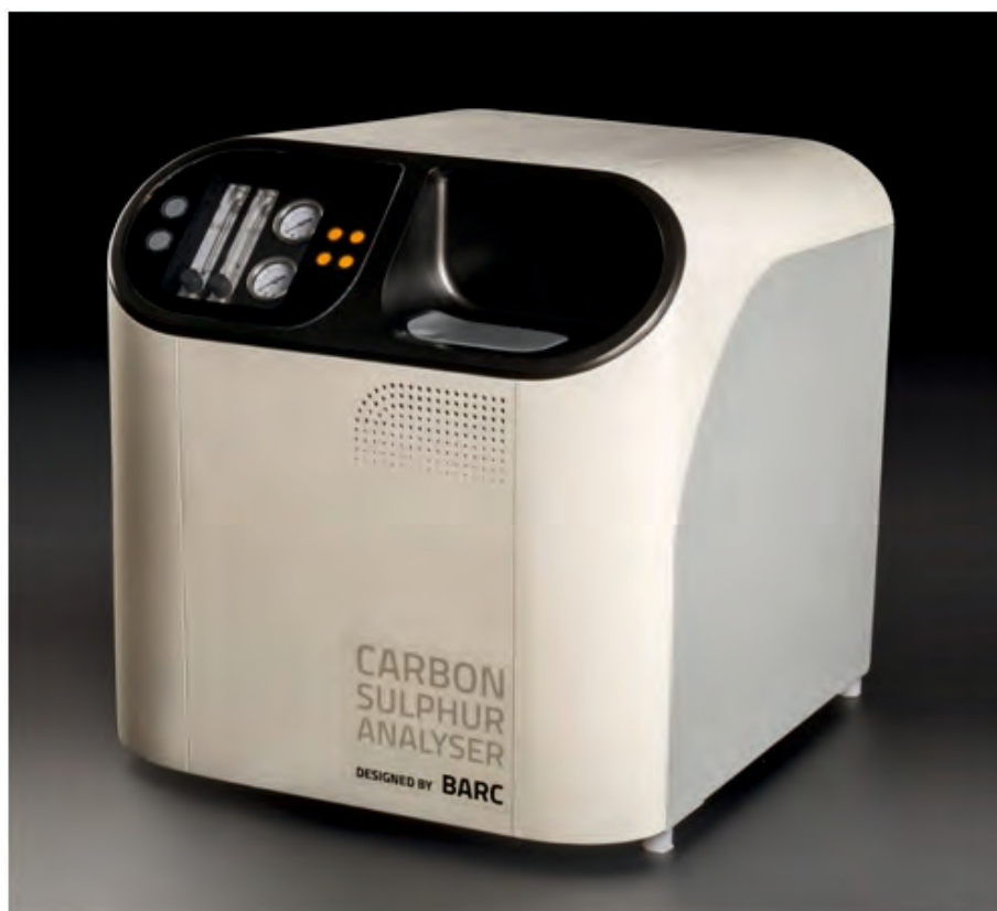
Compact Carbon-Sulfur Analyser developed in BARC
