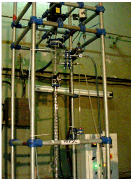
Miniaturized Pulsed Stirred Column setup used for extraction and stripping of Zr from ZNCS
