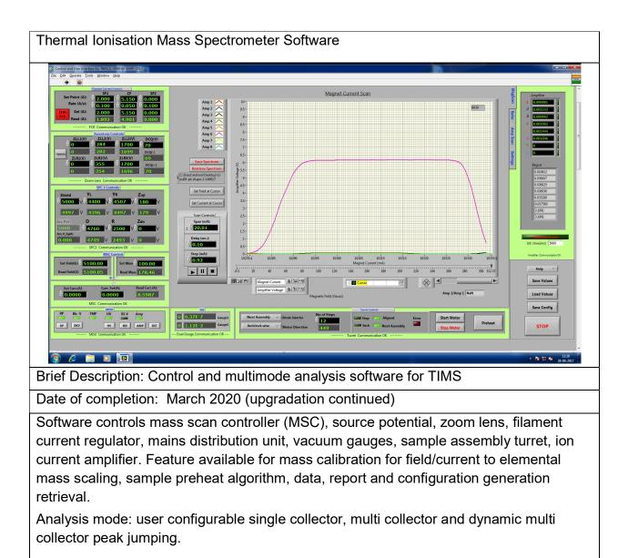
This software is being used in all TIMS, EmA&ID has developed (10 nos.)
