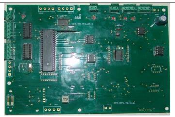
**Brief Description:** Magnetic Field Regulator (MFR) regulates magnetic field of 0 to 1 Tesla in magnetic analyser of magnetic sector Mass Spectrometer. MFR consists of Microcontroller, DAC, OP AMP based IGBT driver, RS232 etc.
