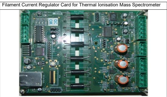
**Brief Description:** This card has been used to control triple filament assembly of Thermal Ionisation Mass Spectrometer (TIMS). It consists of SoC controller, dual DAC, OP AMP based IGBT driver, 10 kV optical isolators, Ethernet controller etc.
