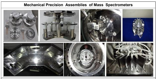
Mechanical design, fabrication and assembly of all the mechanical precision assemblies required for the development of different types of Mass Spectrometers like TIMS, PGMS, MC-ICPMS, RGA, and He-MSLD required for different users of DAE and in house R&D requirements.
