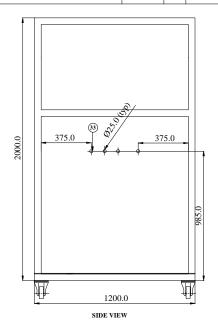
C1: ASSEMBLY LAYOUT OF CAPACITOR BANK IN RACK-2
