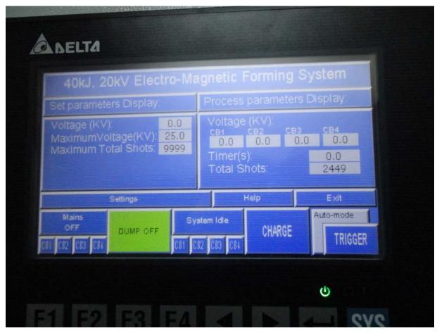
Fig 2.3: Screen is the main operational Screen of the HMI
