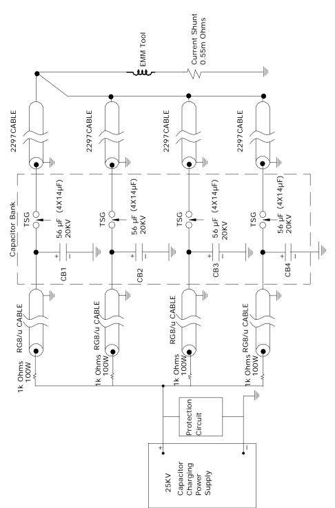
A3: Wiring Connection Diagram of Power Supply, Capacitor Bank and EMM Tool
