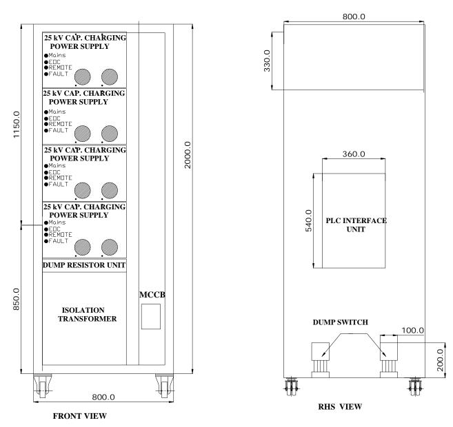
B1: Assembly Layout of Power Supply, PLC Controls and Dump Switch in Rack-1
