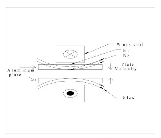
Fig. 2.5 Coil current and magnetic field
