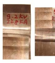
Fig 5.8 Cu -Cu sheets EM welded
