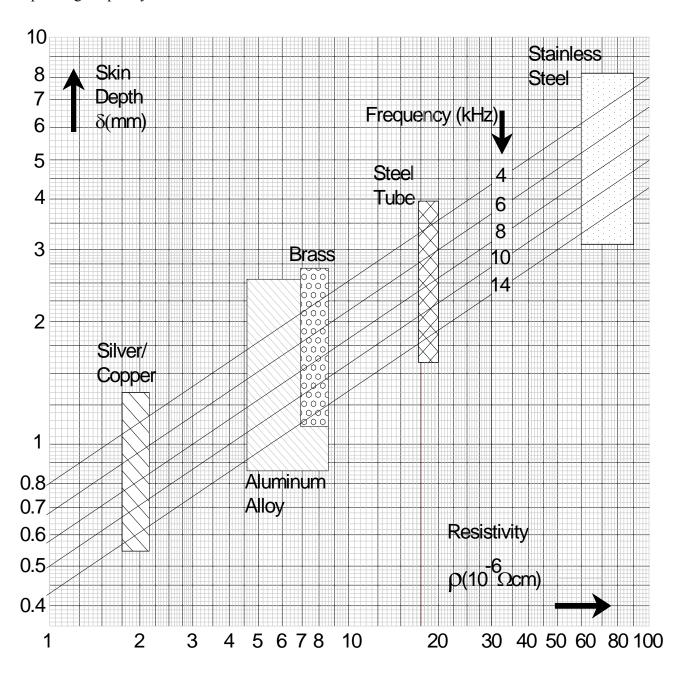
Fig. 2.4 Chart for skin depth vs electrical resistivity of most common materials at various operating frequencies. [7]
