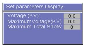
• In the process parameters, process voltages of four capacitor bank modules, viz: CB1, CB2, CB3, CB4 are displayed as shown below. The timer (s) indicator gives the processed charging time in seconds. The total shots indicator display the cumulative number of shots taken upon the capacitor, its value is stored irrespective of the system is switched ON or OFF.
