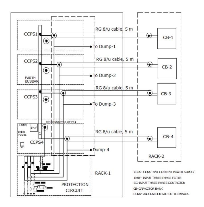
A4: High Voltage interconnection diagram between power supply and capacitor bank
