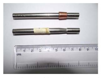
Fig.5.13 Joined samples of the D9 clad to SS316L end plug
