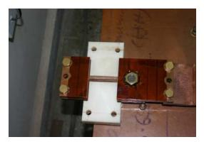
Fig 5.5. EM Welding setup for sheet samples Fig 5.6 EM Welding coil for flat sheet to sheet
