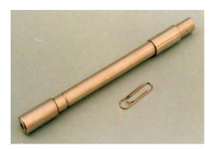
Fig 5.1 Magnetic Flux Concentrator  $\,$  Fig 5.2 Two Al plugs collapsed at two ends of Al rod
