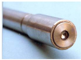
Fig 5.3 Copper lug swaged on Al-multi-core cable Fig 5.4 Al-plug collapsed on SS-rod
