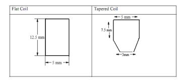
Fig. 2.6 Flat rectangular and tapered cross-section of the coil
