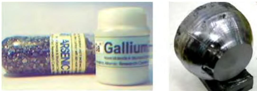
**Fig. 4: (a) 6N Arsenic and 7N Gallium prepared at MAT Lab, BARC, (b) Gallium arsenide single crystal grown at SSPL, Delhi from BARC supplied material (weight ~4 Kg)**
