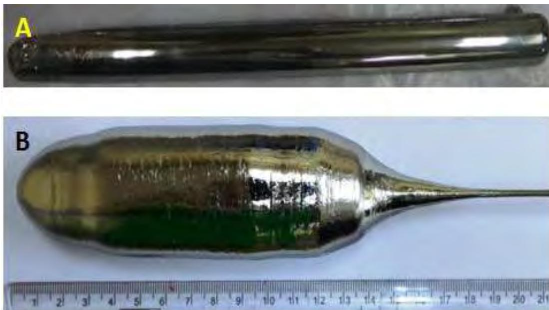
**Fig. 7:** (A) ~8 to 9N pure germanium ingot from Zone-refining unit, and (B) Single Crystal (<100>) of germanium (950 g) grown by TPD from ~8N pure germanium supplied by Chemistry Division.
