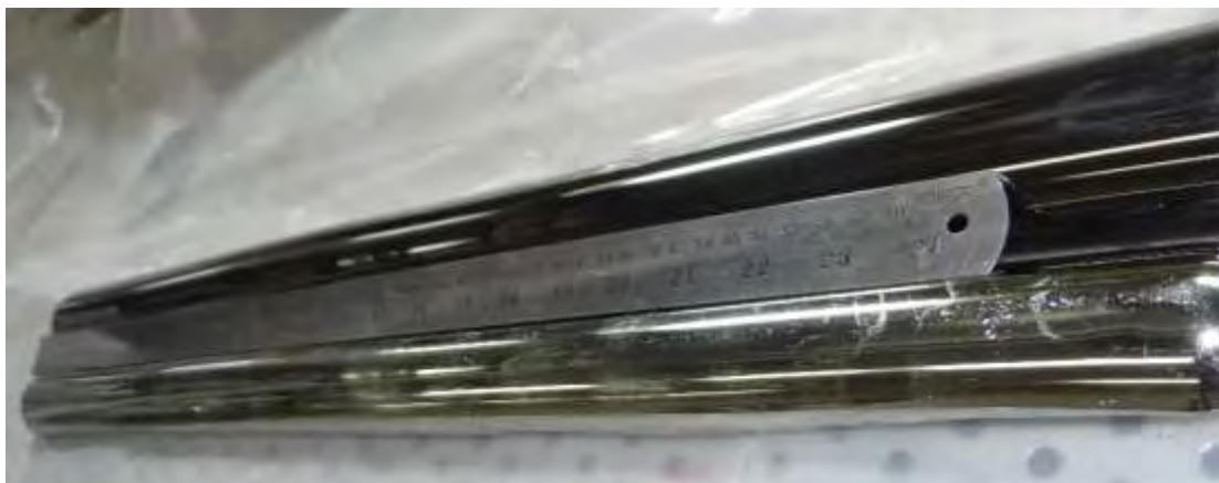
**Fig. 8:** (A) Zone refined detector grade purity germanium ingot.
