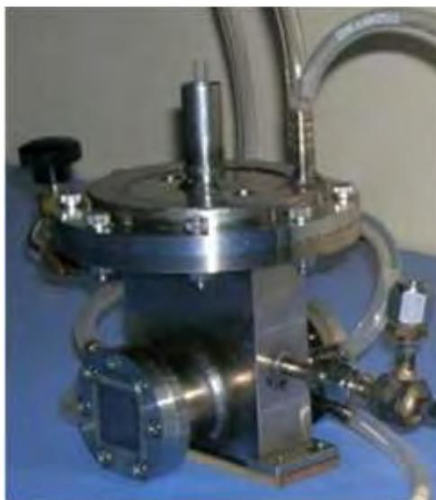
**Fig. 3: A SS-cell equipped with Be-windows for *in-situ* EXAFS study of catalytic materials at EXAFS beam line in INDUS-2 at RRCAT, Indore (developed in collaboration with Applied Spectroscopy Division & CDM)**
