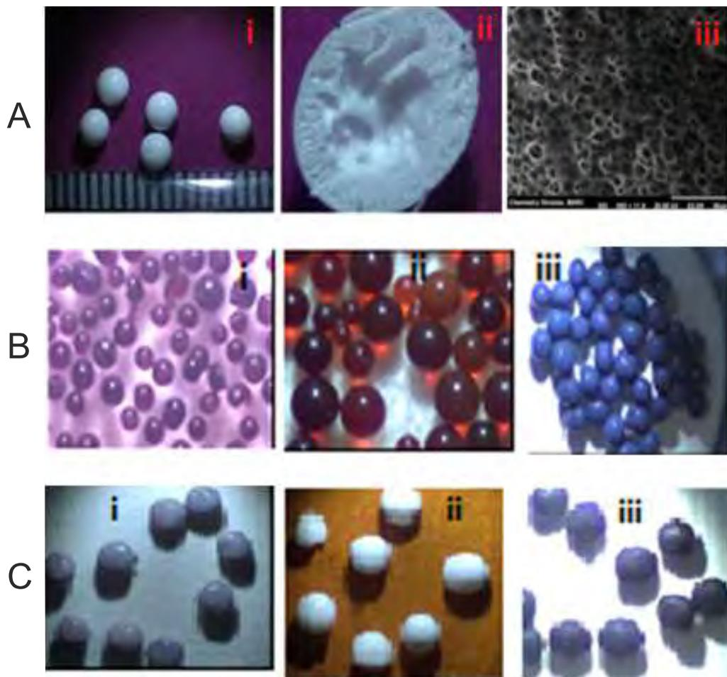
**Fig. 1:** (A) (i) Optical image of D2EHPA-encapsulated polymeric beads for sorption uranyl ions (ii) crosssectional view of the bead (iii) SEM image of the bead (B) Optical images of inorganic sorbent polymer composite beads (i) Resorcinol formaldehyde (RF) bead (patented) (ii) RF-XAD bead (iii) KCoHCF-Gel bead (C) Optical images of inorganic sorbent polysulphone (PS) beads (i) CuHCF-PS composite beads (ii) TiO<sub>2</sub>-PS composite beads (iii) MnO<sub>2</sub>-PS composite beads
