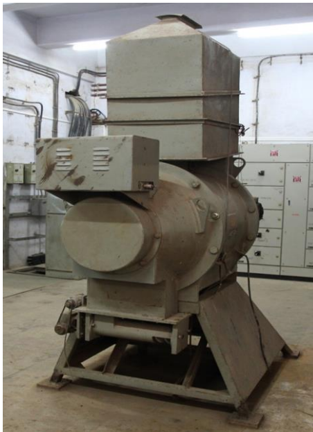
Fig. 1: A dry storage type grain irradiator with grain lifting conveyor system (collaboration with AECL, Canada, currently the facility is not in operational state).
