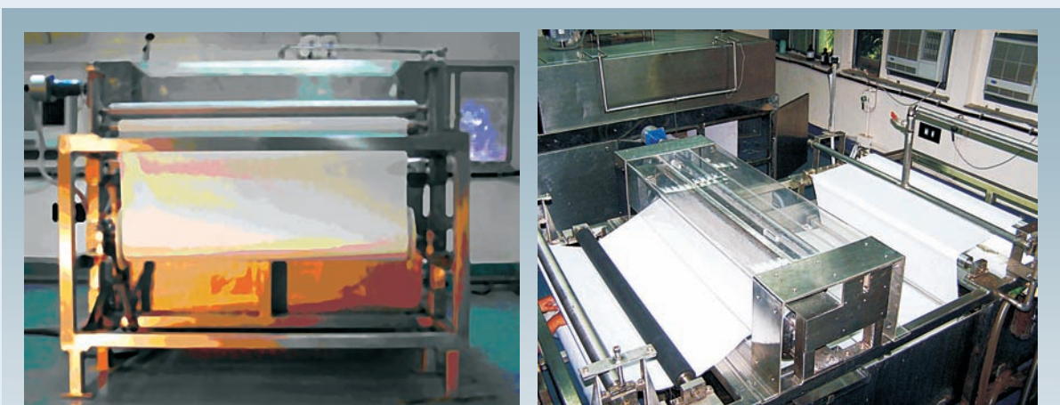
Membrane Casting Machine at BARC
