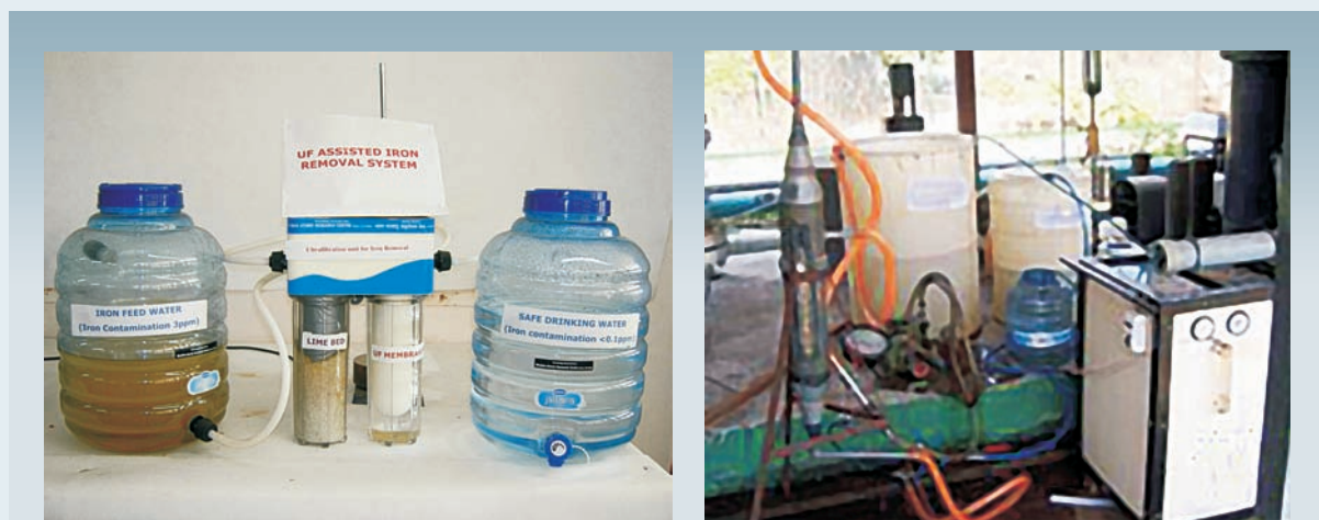
UF Assisted Domestic Size Iron Removal System
