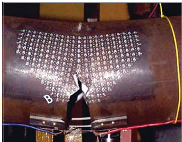
Out-of-plane Crack Growth on 8" Carbon Steel Pipe during Fracture Experiment
