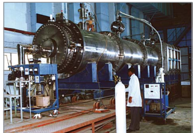
KALI-5000 System (1 MV, 40 KA, 100 ns, 5 KJ)
