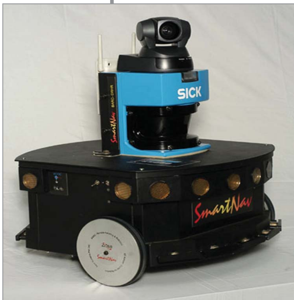
SmartNav: Mobile Robot for Remote Survey & Inspection
