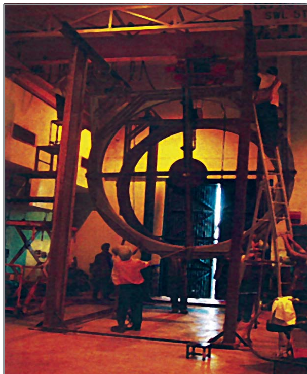
Large Volume Electromagnet for Bending of Strip Electron Beam
