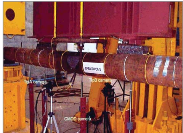
Imaging Set-up for Fracture Experiments to Monitor Crack Growth and Crack Mouth Opening Displacement Installed at S.E.R.C., Chennai
