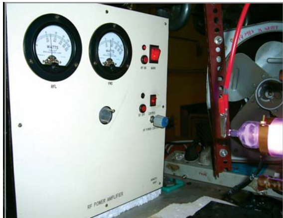
100 MHz 200 W RF Power Supply
