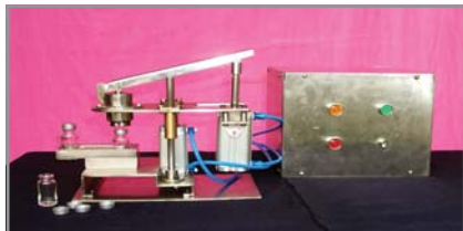
10-ml Vial Crimping Unit Installed in ^{131}\text{I} - Processing Plant
