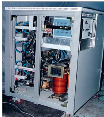
800 A, 10 V Current Regulator for ECR Ion Source
