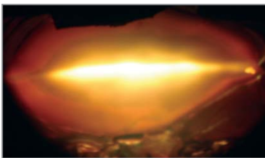
60 KV, 60 KW Electron Beam on Copper (Photo taken with Neutral Density Filters)
