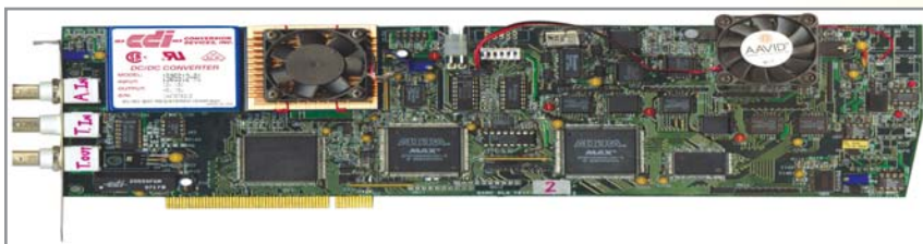
TD1500 – PCI Bus Based 500 MSPS Digitizer
