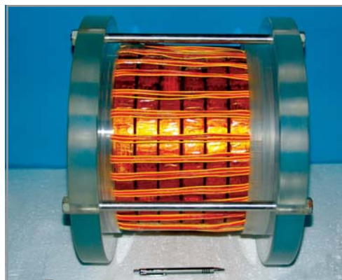
Magnetic Pulse Compression Switch for 20 \mu s/5 \mu s
