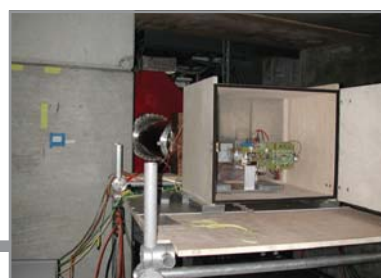
Two PACE2a Test Boards Operating Synchronously in PSI Beam
