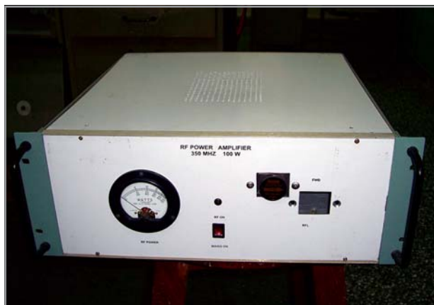
350 MHz 100W Driver for Klystron
