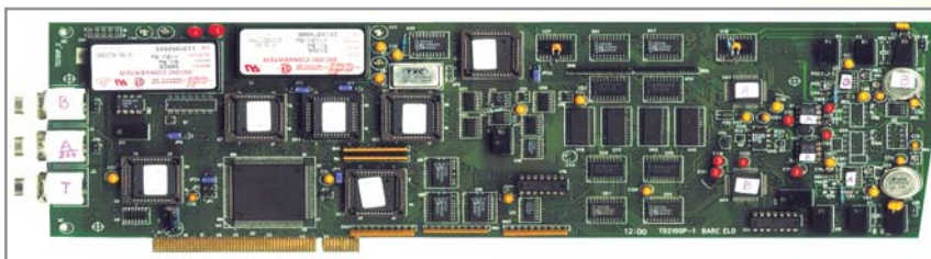
TDP 2100P PCI Bus Based 200 MSPS Digitizer
