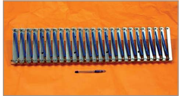
750 KV Resistive Voltage Divider Module
