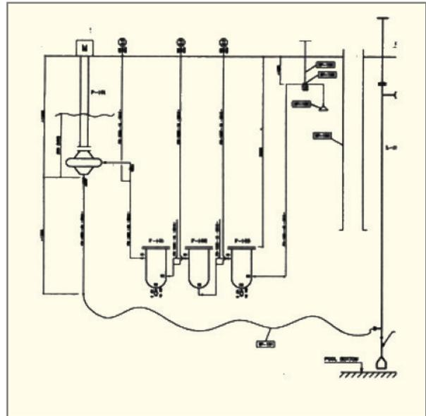
Schematic of the water filtration system
