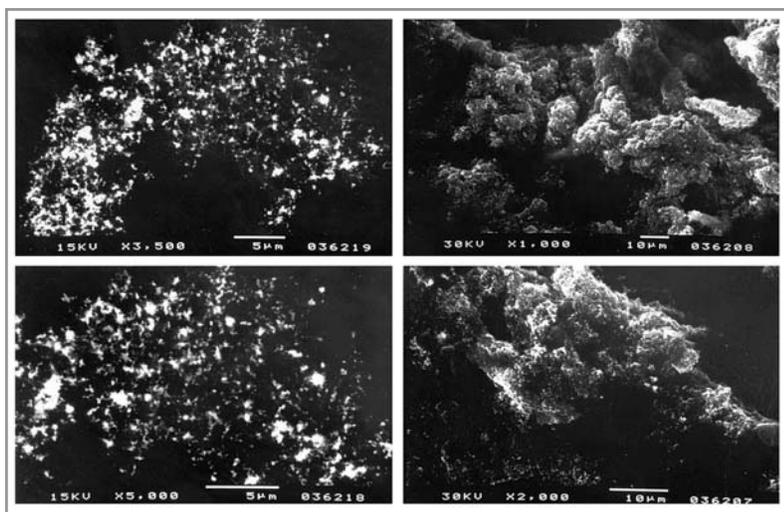
SEM micrographs of Zn aerosols produced using PTAG
