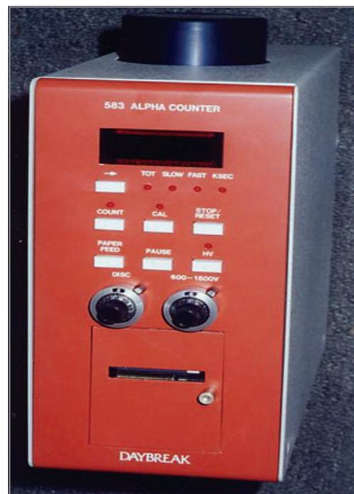
Gross alpha Counter with Pairs Technique, routinely used in BARC for determination of dose rate.
