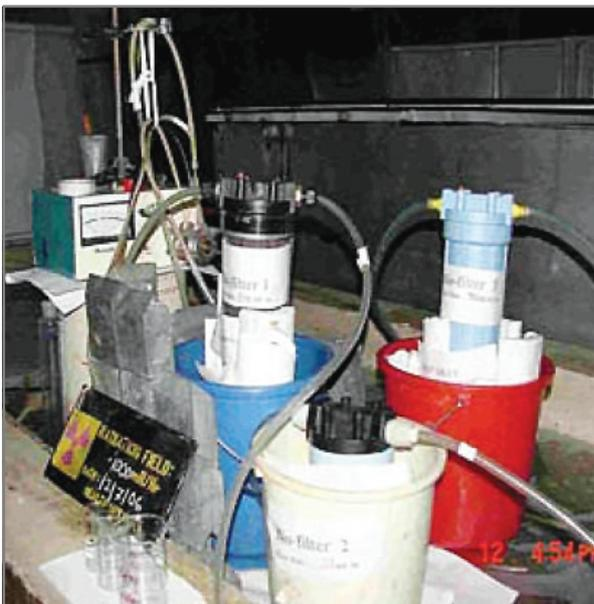
Set up using 3 filters
