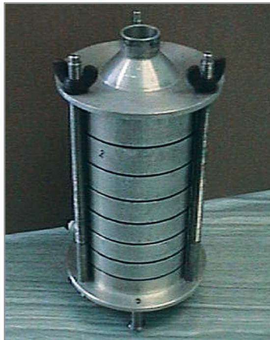
Assembled view of Particle Aerodynamic Size Separator
