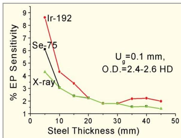
Comparison of Sensitivity Achieved For Radiography of Steel Using Different Sources
