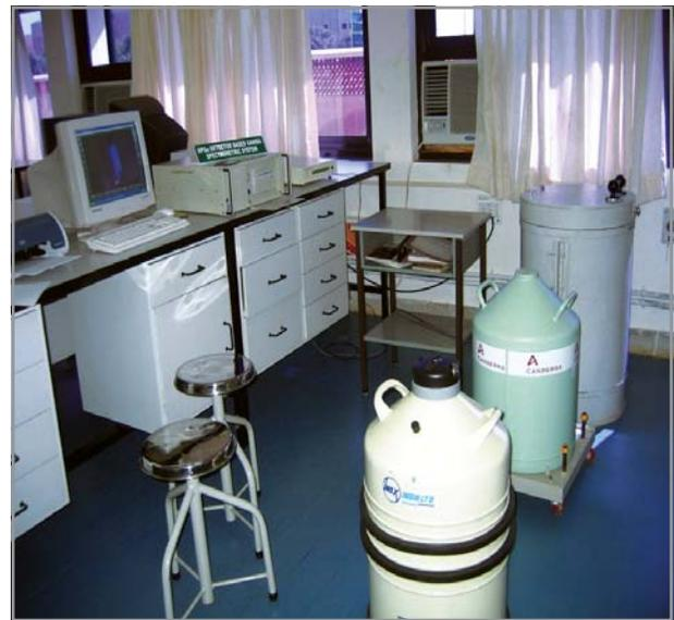
HPGe Detector Gamma Spectrometry
