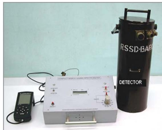
PCGS System with its detector in an enclosure and GPS receiver
