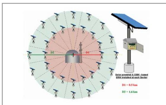
Environmental radiation monitoring network along with the solar powered radiation monitors
