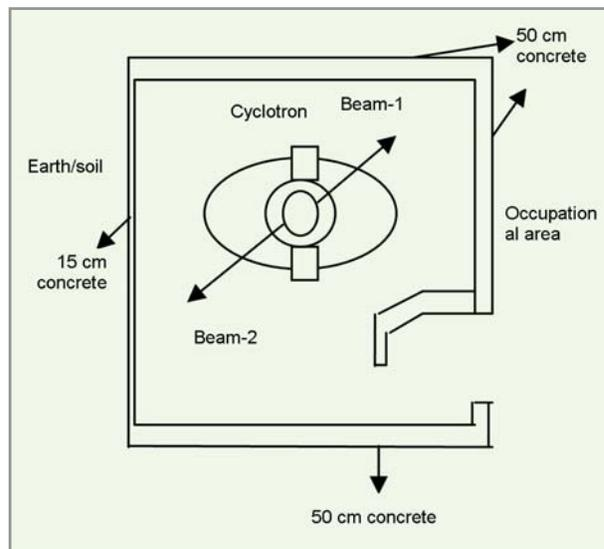
Block diagram of self-shielded cyclotron facility showing dual beam direction
