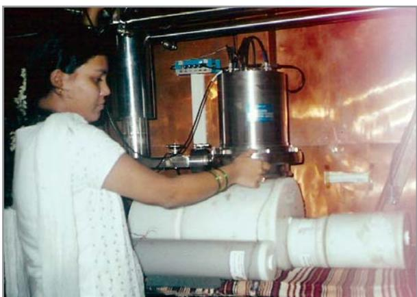
Steel room whole body monitor showing Phoswich detector and IAEA BOMAB phantom in position
