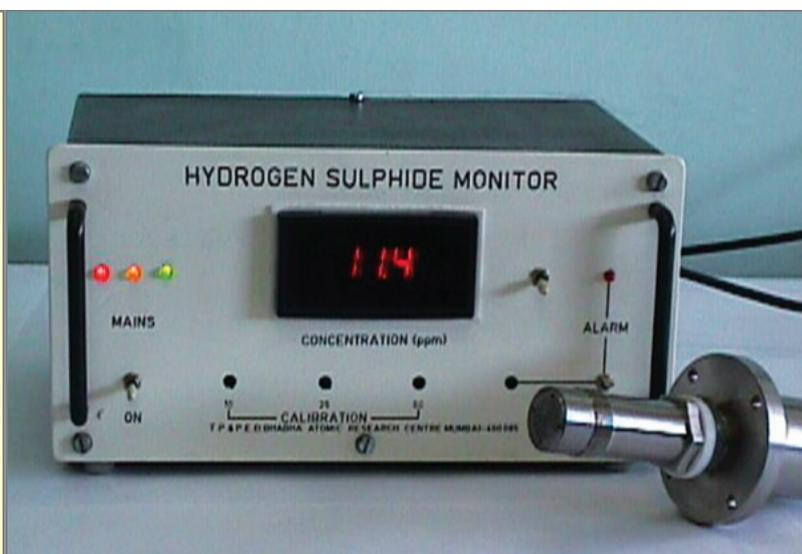
$\text{H}_2\text{S}$  sensor with electronic display unit
