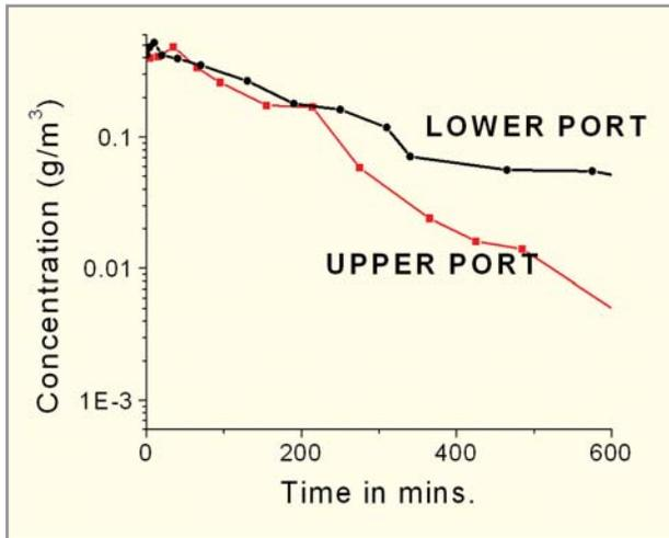
Observation of aerosol stratification at two heights of the vessel
