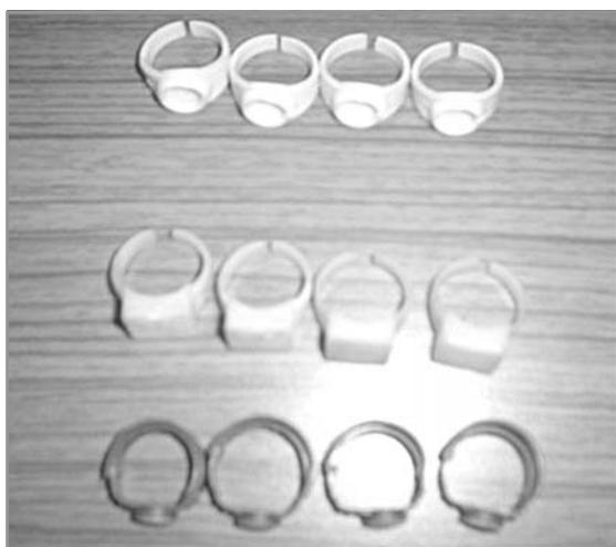
Different designs of Finger Ring dosimeters
