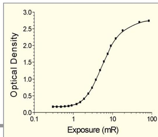
X-Ray sensitometric curve of Medical X-ray film
