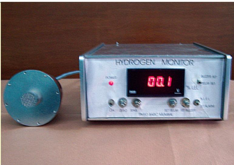
Hydrogen sensor with electronic display unit
