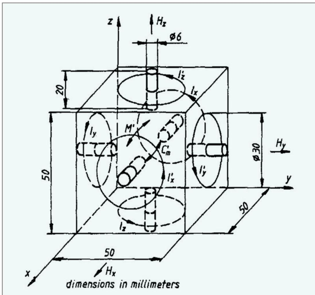
Six-face arrangement of dipole and loop antenna elements
