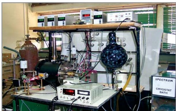
Flash photolysis resonance fluorescence machine
