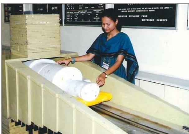
Shadow shield bed whole body monitor with IAEA BOMAB phantom in position
