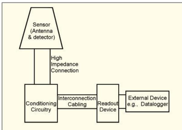
Main building blocks of the RF radiation monitoring instrument
