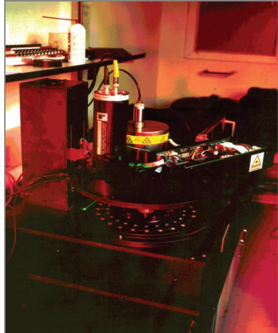
TL/OSL system routinely used in BARC for luminescence dating applications.
