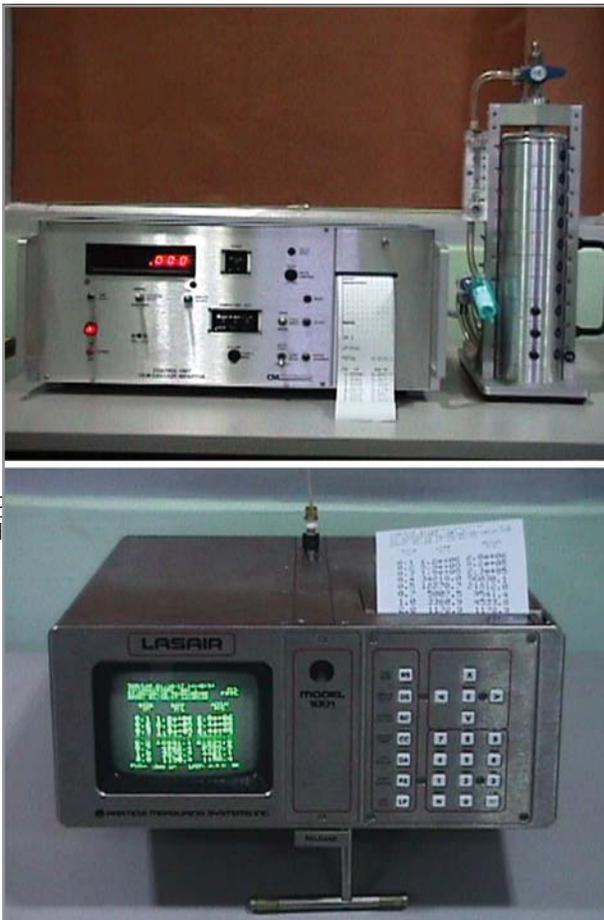
Photograph showing: (a) Quartz-crystal microbalance cascade impactor (b) Optical particle counter
