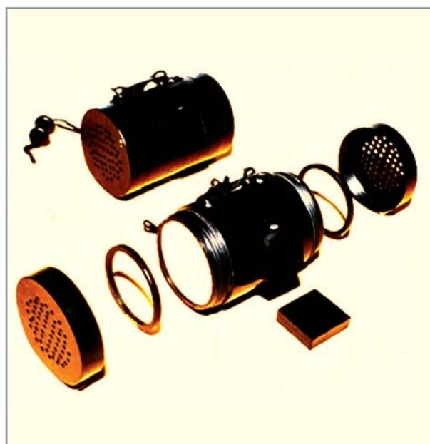
Twin Cup radon/thoron dosimeter
