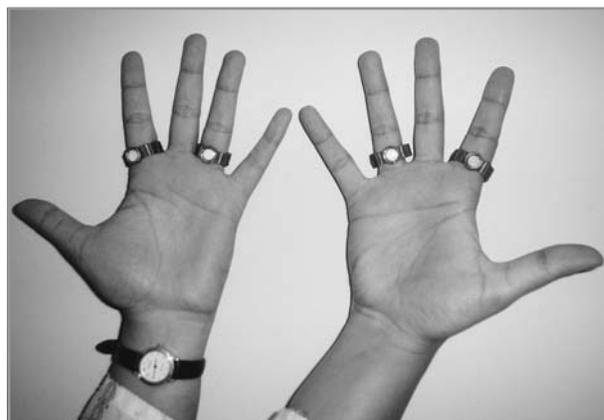
A palm showing the Finger Rings with dosimeters
