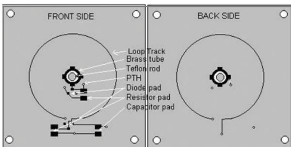
PCB layout for electric dipole and magnetic loop antenna
