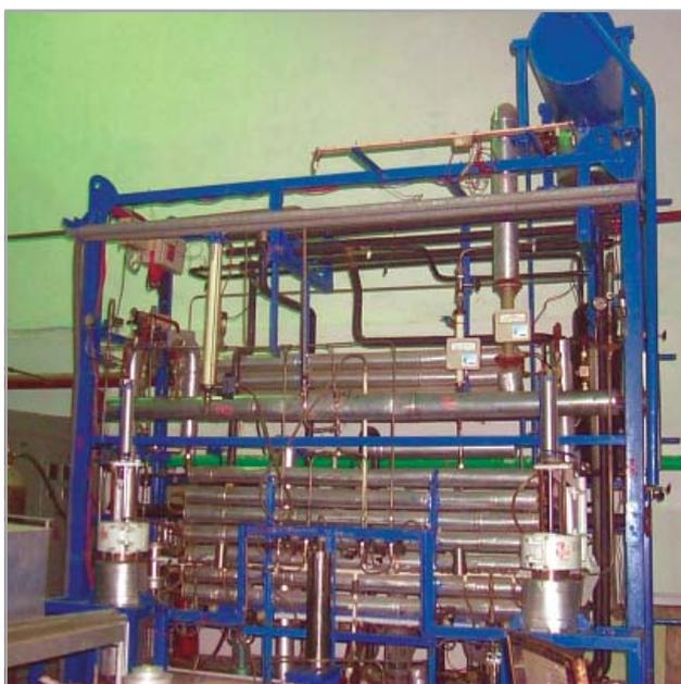
Supercritical fluid extraction pilot plant
