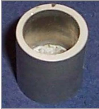
Photograph of a glass-to-metal seal fabricated using Al as outer body.
