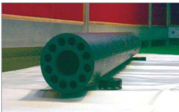
Prototype hot channel tube for CHTR
