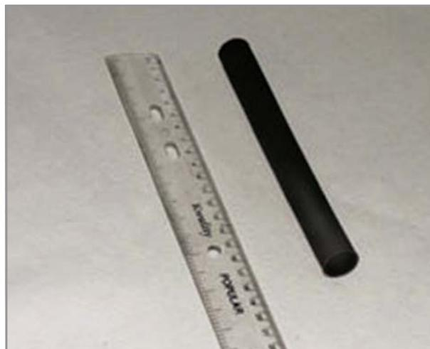
Porous sintered LSM cathode tube
