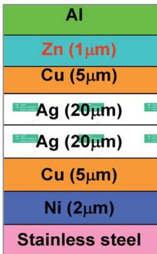
Compatible multilayers for diffusion bonding of stainless steel to Aluminium
