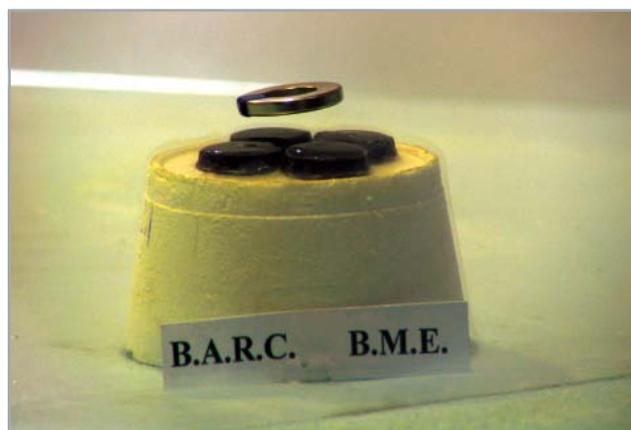
Photograph showing levitation of a small magnet over a set of four pellets
