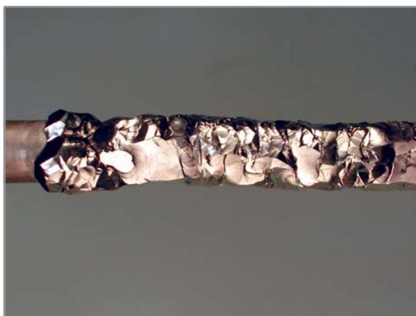
Macrostructure of a section of crystal bar zirconium
