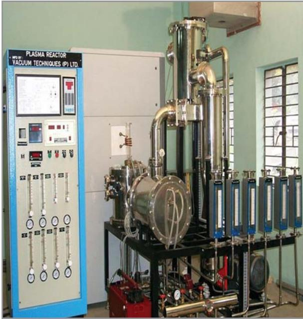
4 MHz 50 kW RF Plasma Reactor
