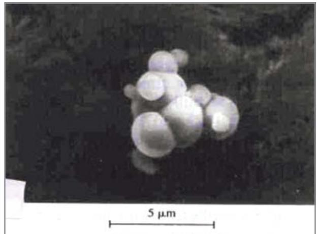
Sulphate route Morphology of precursors for alumina by homogeneous precipitation method
