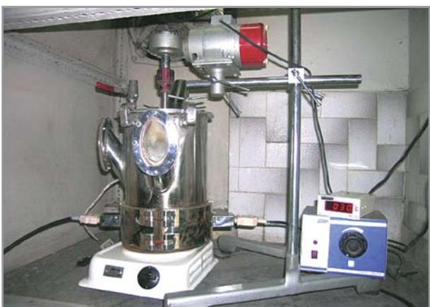
Set up for combustion synthesis
