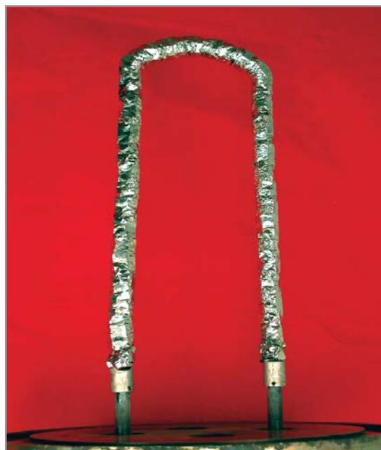
Crystal bar zirconium with the retort cover flange
