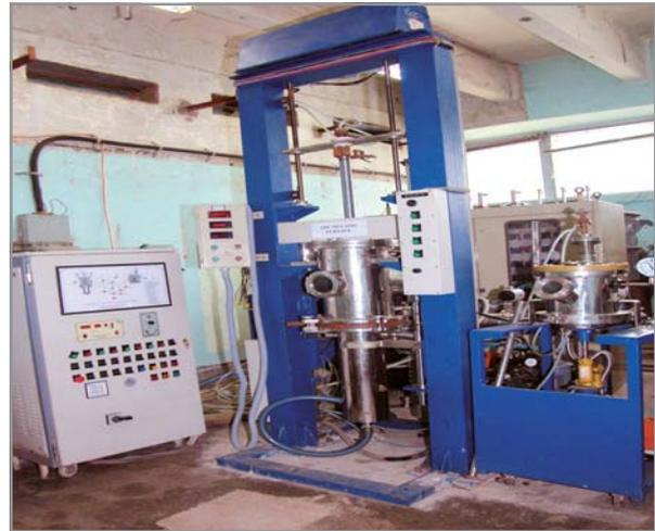
Vacuum arc melting furnace
