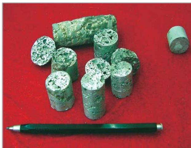
Aluminium foams formed using Titanium or Zirconium hydrides
