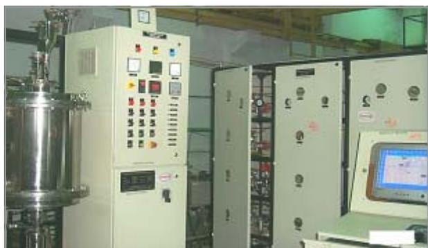
High temperature fluid/spout bed furnace
