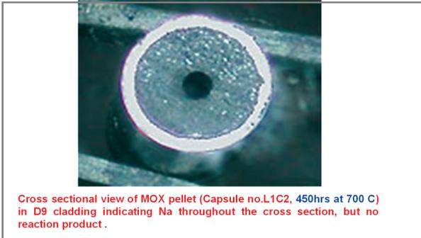
A fuel pin undergoes thermal cycling during power ramp or shut down/restart of a reactor. Any second phase precipitation may lead to dimensional changes which is undesirable.
