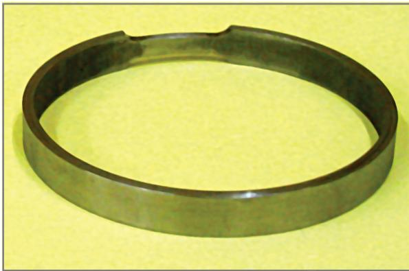
Ring Tension Test Specimen
