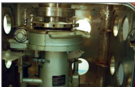
Installation of Rotary Press in the New Glove Box Line for PFBR
