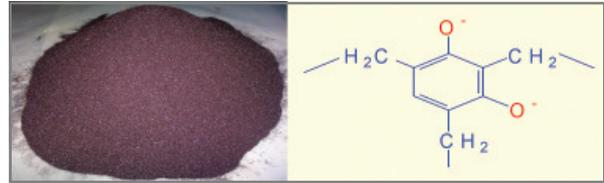
Resorcinol formaldehyde polycondensate resin (RFPR) showing Cs-selective phenoxide ion exchange sites
