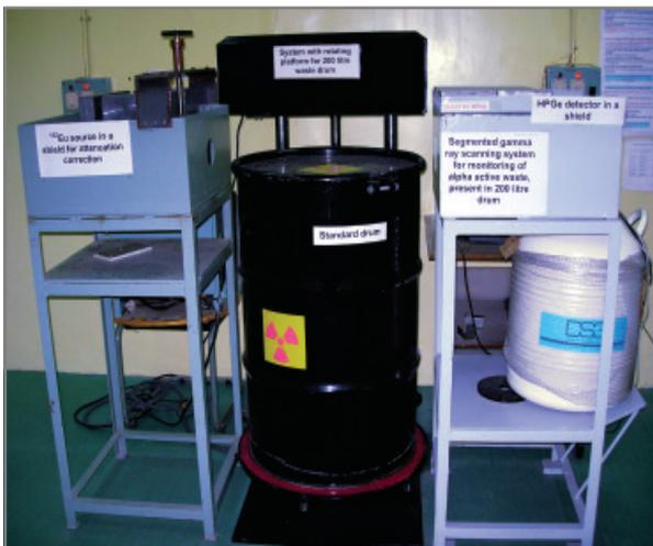
The gamma rays spectrum analysis is carried out using computer program based on digital signal processing developed in-house. The  $^{239}\text{Pu}$  activity above 25 mg can be detected in a 200-litre drum. The detection limits will go up in the presence of gamma ray background or high-density materials. A safe estimate can be above 50 mg of  $^{239}\text{Pu}$ .
