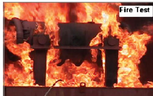
the cask design. Two double bundle PHWR fuel transport cum storage casks of modified design has been fabricated.
