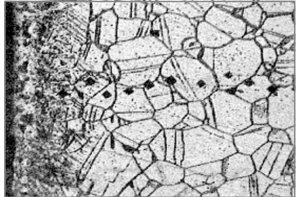
Photomicrograph of SS-316 (20%CW) showing pellet/clad interface and Vickers indentations after fuel-clad-coolant compatibility experiment
