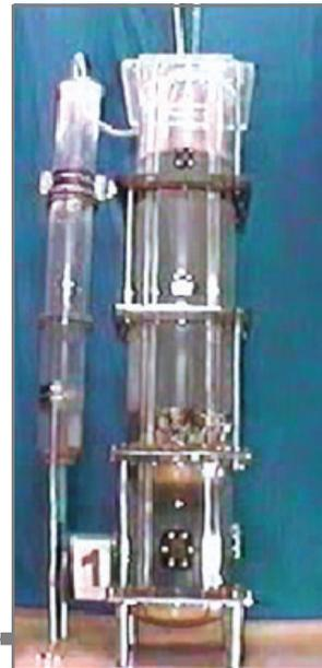
Hydraulic Pulse Dissolver Scale-Up Model
