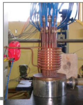
Laboratory scale cold crucible melter
