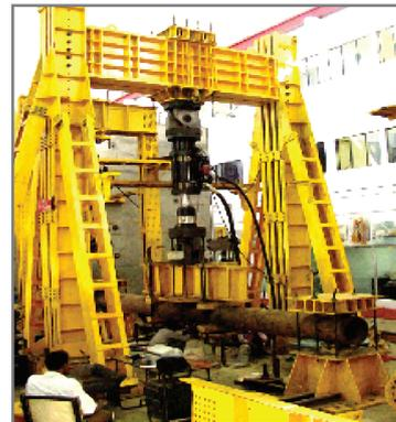
Fatigue Test of PHT Piping
