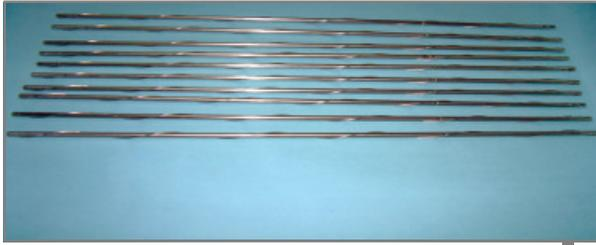
MOX Fuel Pins for PFBR Experimental Sub-Assembly
