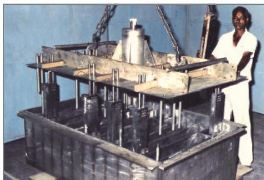
KARP Integrated Spent Solvent Treatment Unit of 200 LPH capacity
