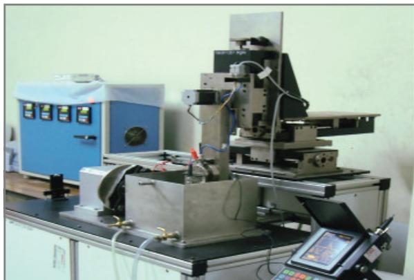
Ultrasonic Weld Scanning System for PFBR End Plug Welds
