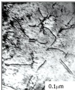
Defect Structure In Irradiated Zircalloy-2
