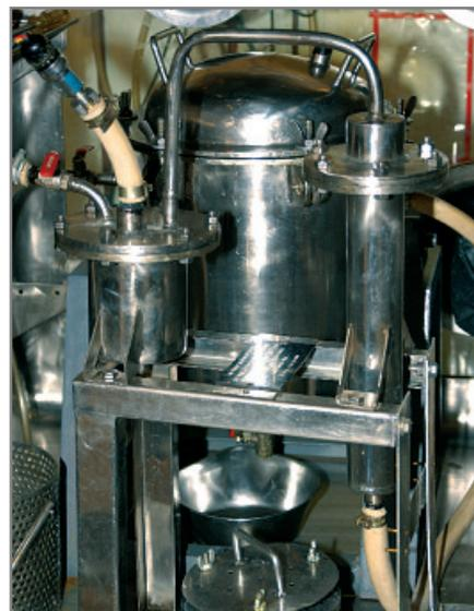
Impregnation Set-up Inside the Glove Box
