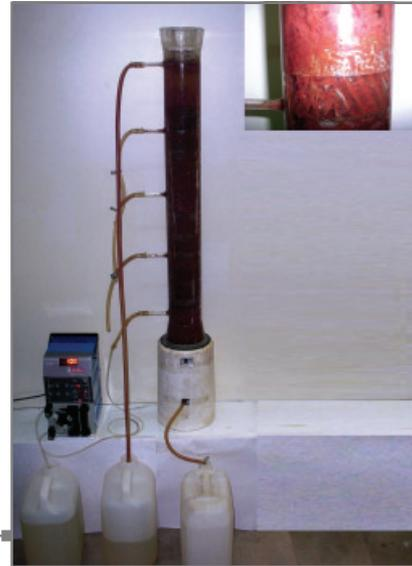
Upflow column bioreactor for denitrification (inset showing biomass attached to porous support within the column)
