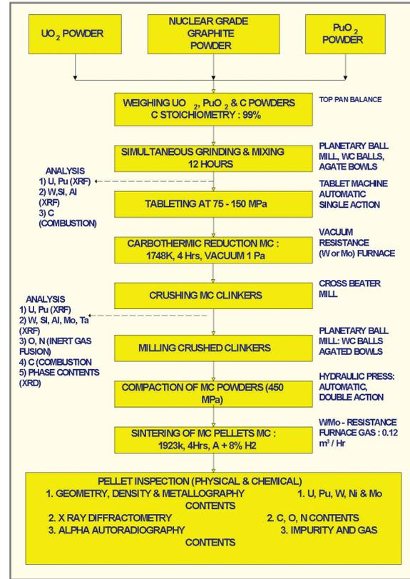
(U<sub>0.3</sub>-Pu<sub>0.7</sub>)C mixed Carbide fuel pellet fabrication flow-sheet
