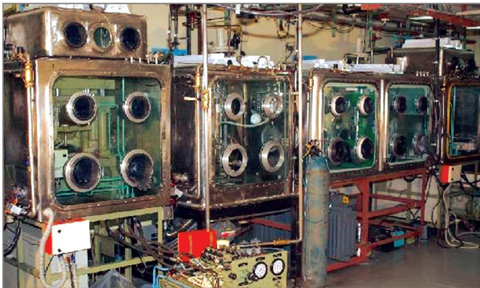
New laboratory facility being set-up for FBTR fuel pin production
