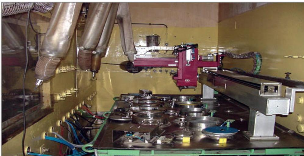
Automated Metallographic Sample preparation system in Hot Cell
