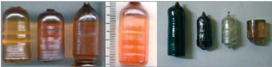
Some of the crystals that have been grown using crystal pullers.
