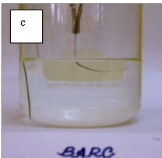
Photographs of actuator action, (a) before application of voltage and on application of (b) +2 V and (c) -2V voltage.
