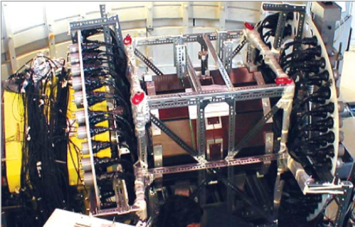
A new detector, ENSTAR which has been constructed at BARC and assembled at Juelich for this purpose. This detector consists of 122 scintillator elements each with wavelength shifting optical fibers connected to photo-multiplier tubes. The construction, installation, offline and in-beam testing of the detector was completed in 2004.
