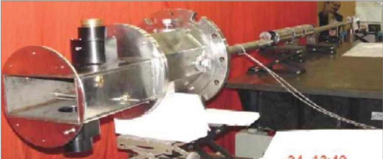
A periscope 5.3 meter in length fabricated for remote controlled Fast Breeder Test reactor (FBTR). Lenses  $L_{1A}$ ,  $L_{1B}$  and  $L_{1C}$  form the zoom lens objective of the periscope.
