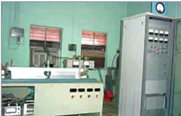
Slab type RF excited Carbon dioxide laser system
