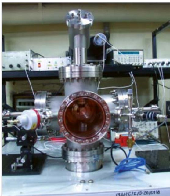
Photograph of the supersonic free-jet-laser induced fluorescence setup.
