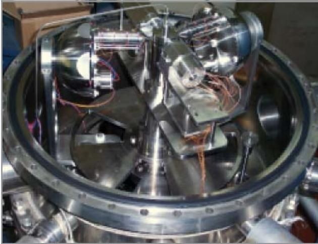
High Resolution Electron-Optic Spectrometer and test spectrum recorded for  $N_2$ . The FWHM is  $\sim 0.5$  eV.
