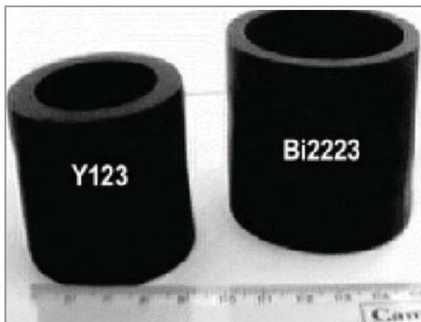
Sintered HTSC oxide cylinders.
