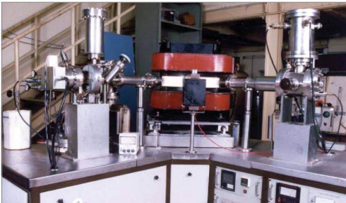
The process gas mass spectrometer
