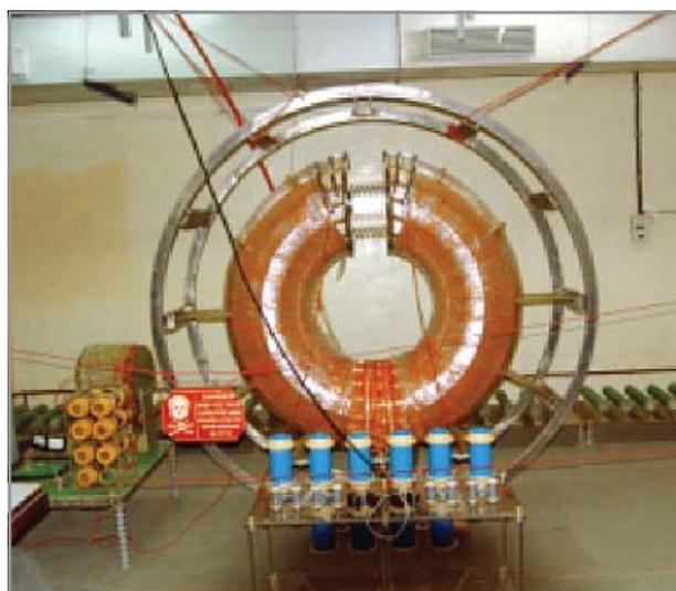
150-0-150 kV, 10 MVA Air cored transformer
