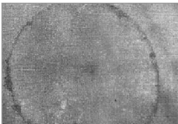
SEM photomicrograph of the same clad surface after exposure to a single pulse of the laser (50X)
