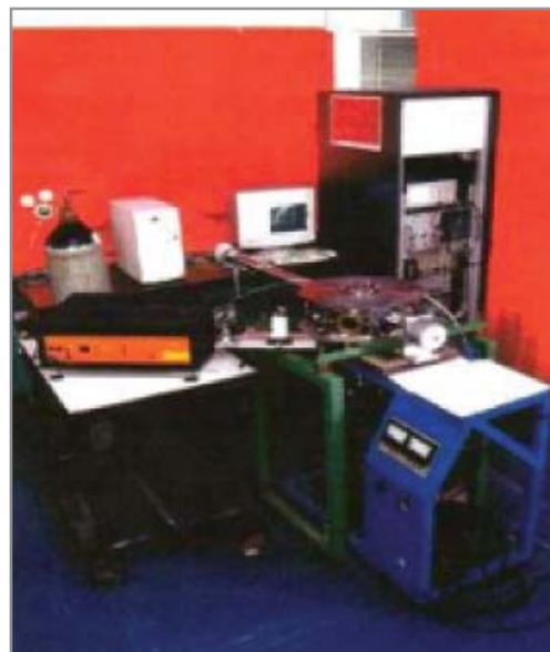
Matrix assisted laser desorption ionization time of flight mass spectrometer.
