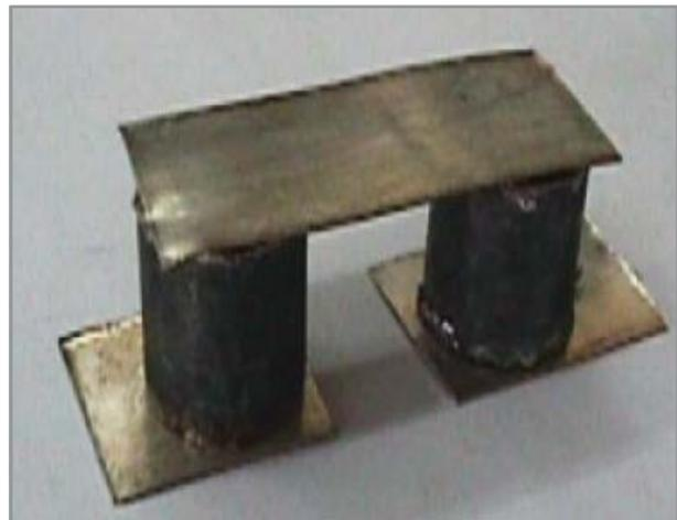
A device consisting of a pair of thermo-elements with a power output of 750 mW.
