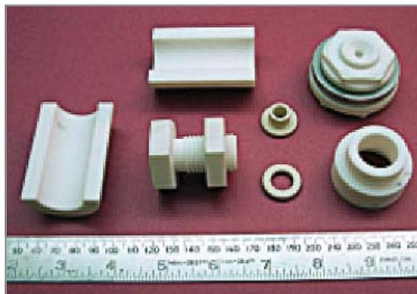
Some of components fabricated from machineable MAS glass-ceramics.
