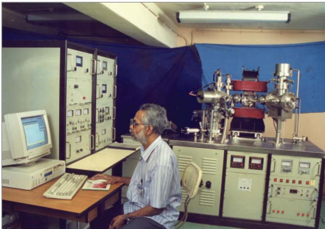
Thermal Ionization Mass Spectrometer
