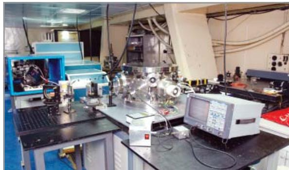
Laser plasma interaction chamber fitted with various diagnostics
