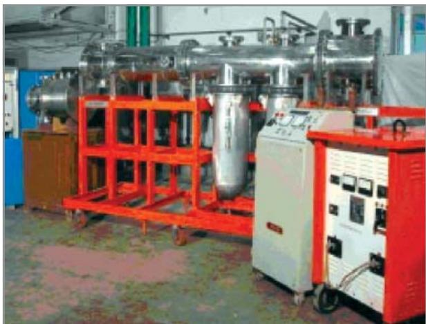
200keV, 5kA, 10-100Hz, 50ns Linear Induction Accelerator.
