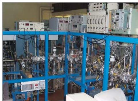
Beamline connected to Electrostatic Ion Trap
